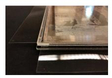
Stratigraphy of the package: borosilicate glass - spacer with plate sitting in its z-trays - borosilicate glass, before trimming Mylar®
