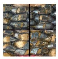
The white areas in the X-ray image of the figure on the left are metal threads used to highlight the figure. On the right are photomicrographs of the metal threads, silver-gilt (upper) and silver (lower) strip wrapped around a silk core magnified n 100x. The details are from the headscarf and dress of the figure, shown front and back.
